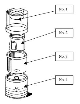
**No. 1--Cover with Filling Opening** The filling opening in the middle of the cover allows you to add ingredients without stopping the machine.
